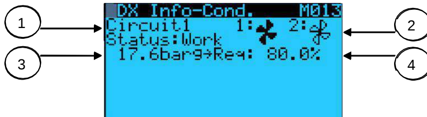
Figure_7.3 Main monitoring page 5 - Condenser fan statuses
