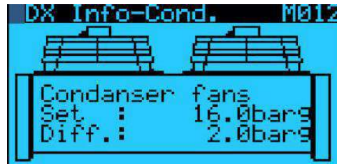
Figure_7.6 Main monitoring page 4 - Condenser fan set
